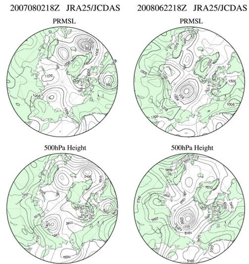
Figure 1: Pressure Fields for Case 1 and Case 2 of PRMSL (hPa, top row) and 500 hPa height (bottom row) for Case 1 (left hand column) and Case 2 (right hand column).
