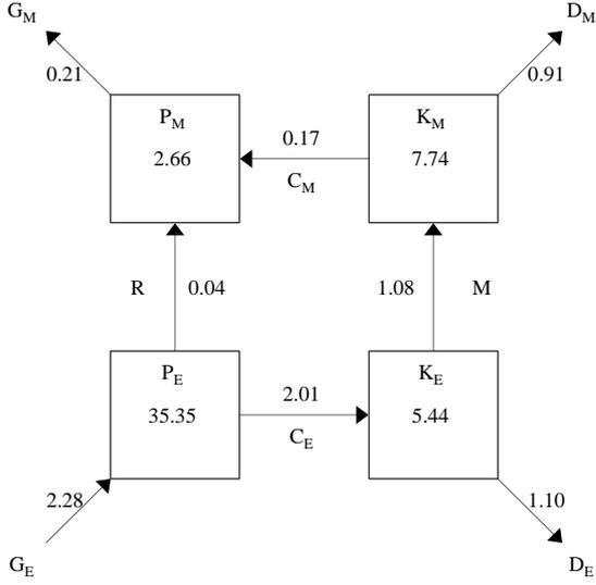
Figure 2: The kinetic and available potential energy cycle for the barotropic and baroclinic components of the Northern Hemispheric atmosphere. The units of the energy are  $10^5 \text{J/m}^2$ , and those of the interactions term are  $\text{W/m}^2$ .
