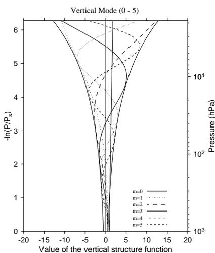
Figure 1: The vertical profiles of the analytical vertical structure functions for  $m = 0 - 5$ .
