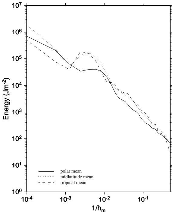
Figure 3: The kinetic energy spectrum in the vertical mode domain. Solid, dotted, and dashed lines are for polar region, mid-latitudes, and the tropics.
