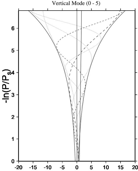
Figure 1: Analytical vertical structure functions for vertical modes  $m$  from 0 to 5.
